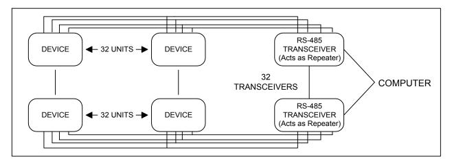
Figure 4.8: 4-Wire RS-485 Communication Installation Connection with Transceiver
